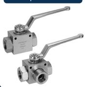
Body Sizes - 06 - 50 Thread Sizes - 1/4" - 2" Thread Forms -BSPP, NPT, SAE, METRIC Pressure Rating -350 - 500 bar | 5075 - 7250 psi Material - Carbon Steel Plating - Trivalent
